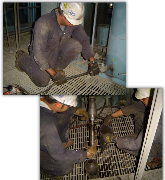
Figure 3: Storm team performing Dirty Air Testing & collection of coal sample
