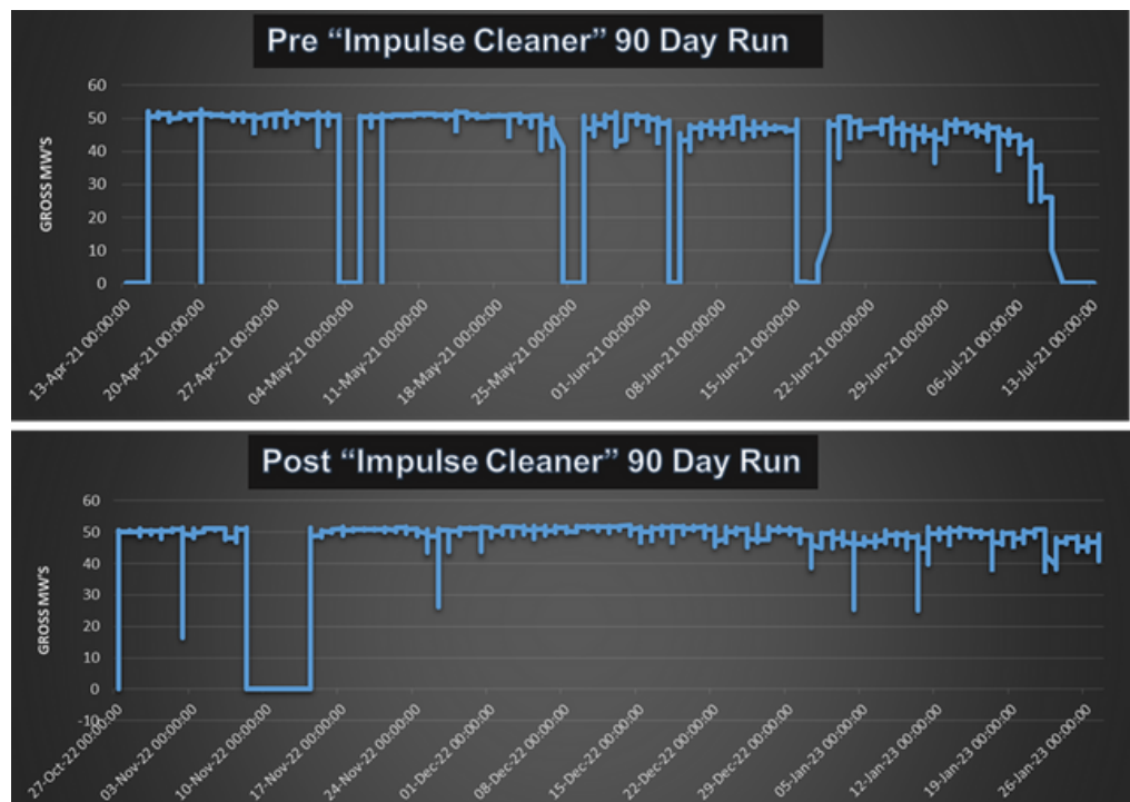
Figure 1: Pre/Post Impulse Cleaner 90-Day Operation to Compare Maintenance Outages
