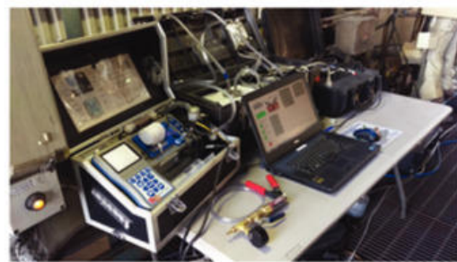
1. The Storm-designed SOAR (Storm Optimization Automated Results) gas sampling system. Courtesy: Storm Technologies
