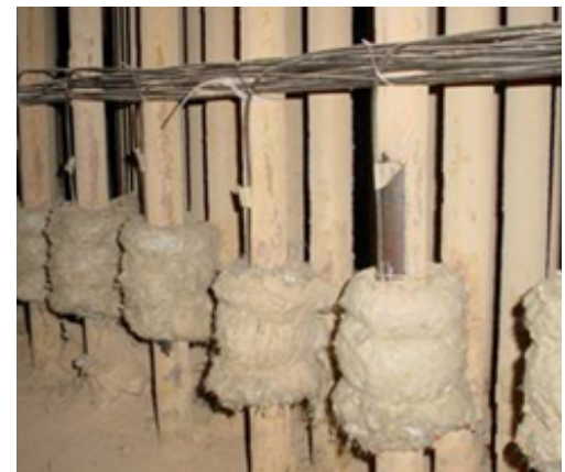
Figure 1: Tube Metal Thermocouples (Left); After Insulation (Right)
