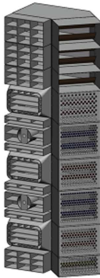
Figure 3: Application of Perforated Plate to help balance secondary air to the individual corners
