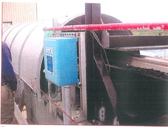
Figure 2. Magnetic separator (typical).
