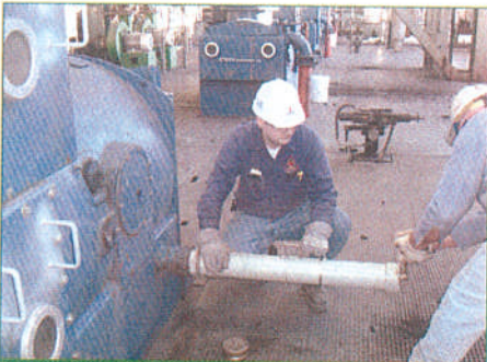
Figure 1. Test personnel coal sampling at the discharge of multiple gravimetric coal feeders during a boiler efficiency test.
