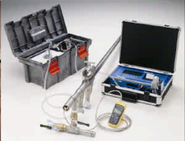
Figure 13 A STORM HVT kit, including a HVT probe, gas sample pump/conditioner and ECOM gas analyzer
