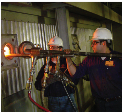
Above: Furnace Exit HVT Testing
