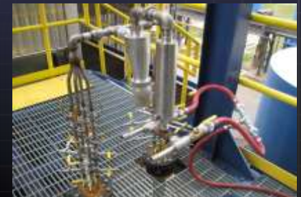
Gas Inlet Test Grid (Temperature, % Oxygen, CO ppm, NO x ppm & Static Pressure)
