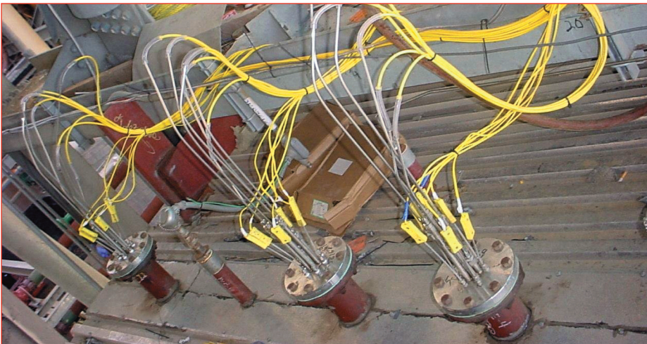
Figure 8. A typical multi-point probe and bubbler grid.
